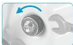
Loosen the 4 transport bolts with a spanner.
