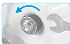
Loosen the 4 transport bolts with a spanner.
